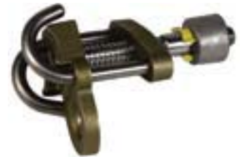
Wire Grip Grips conductor, has hole for block or line hook. WWL for grip is 1,000 lbs (454 kgs) at a 4:1 ratio. 3600 Opening min.5/16" max.7/8" 2 lbs (0.91 kgs) (7.9mm, 2.2cm) 3601 Opening min.1/2" max.1-1/2" 3 lbs. (1.36 kgs) (1.3cm, 3.8cm) Add suffix "U" for Universal, "Q" for Quick Change
