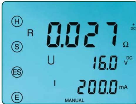
The 4-Point (Kelvin sensing) Bond test shows lead connections, bond resistance test results, test voltage and current.
