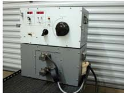
Multi-Amp CB-845 circuit breaker test set following calibration and certification.
