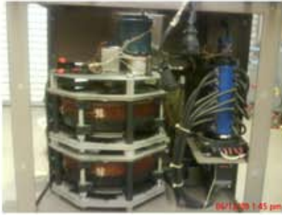
EIL BTS-1000 high current test set. Repairs included Binary Coding Unit plus calibration and certification.
