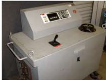
AVO DDA Series Circuit Breaker Test Set - repaired, calibrated and certified.
