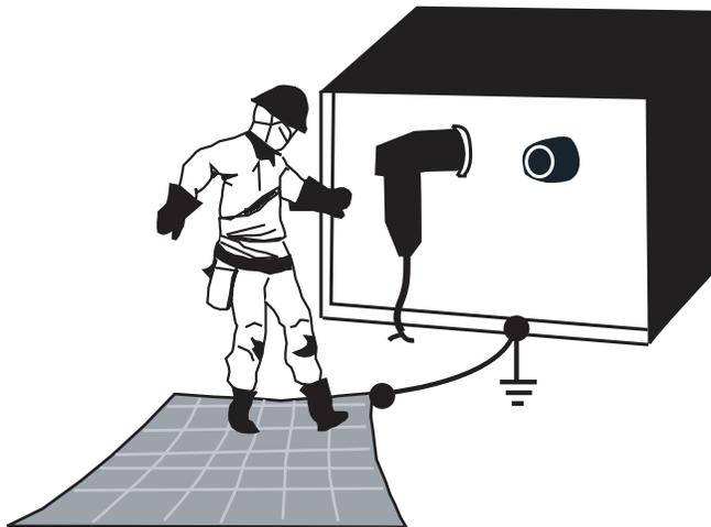
**Use of a Conductive Mat to Develop an Equipotential Zone**
